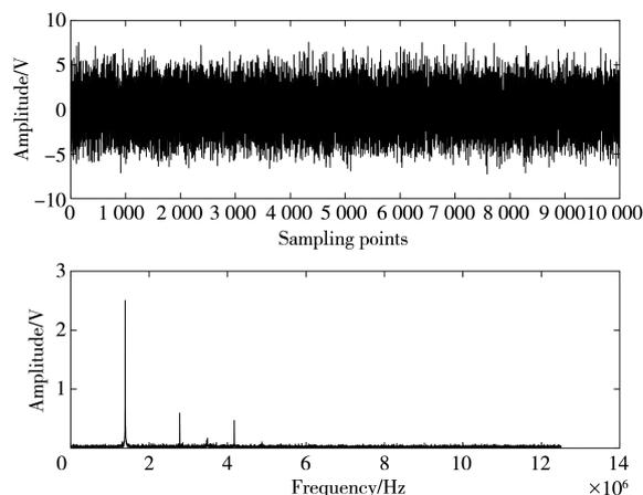
Fig. 6 Time domain waveform and spectrum of noisy signal
