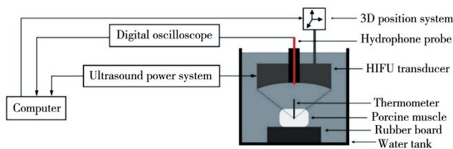
Fig. 5 Experiment equipment
