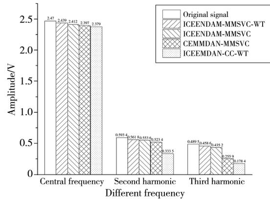
Fig. 9 Comparison of signal amplitudes after four denoising methods
