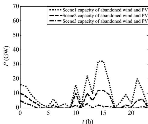
**Fig. 10** Capacity of abandoned wind power and PV power at every time scale in different scenes
