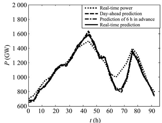
Fig. 8 Predicted curves of load power at different time scales
