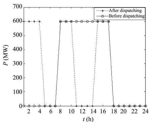
Fig. 4 Outputs of high-energy enterprise load before and after dispatch
