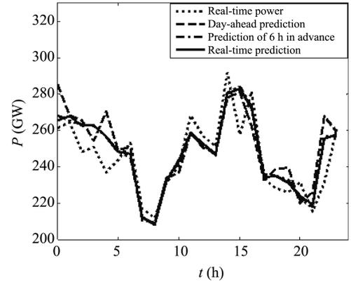
Fig. 6 Predicted curves of wind power at different time scales
