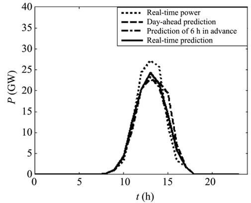
Fig. 7 Predicted curves of PV power at different time scales
