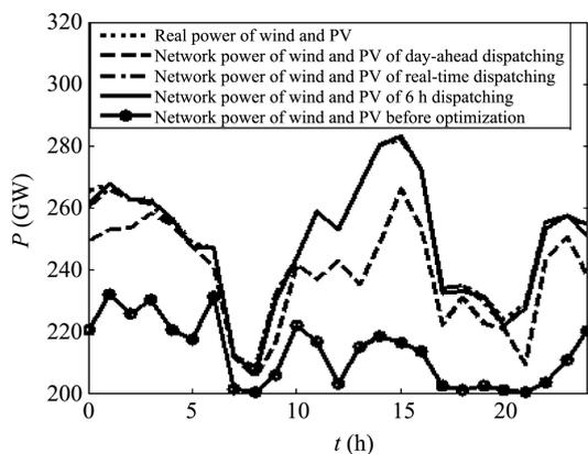
**Fig. 9** Contrast curves of networked wind power and PV power at each time scale
