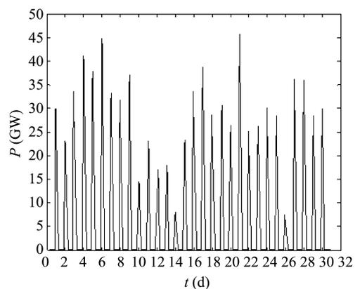
Fig. 3 Monthly output distribution of PV power station
