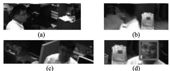
Fig. 10 Head tracing for front-face detection: (a) Side-head, (b) Back-head, (c) Hang-head, (d) Front-head
