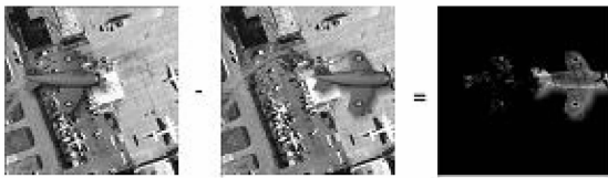
Fig. 1 Motion object detecting using difference of image
