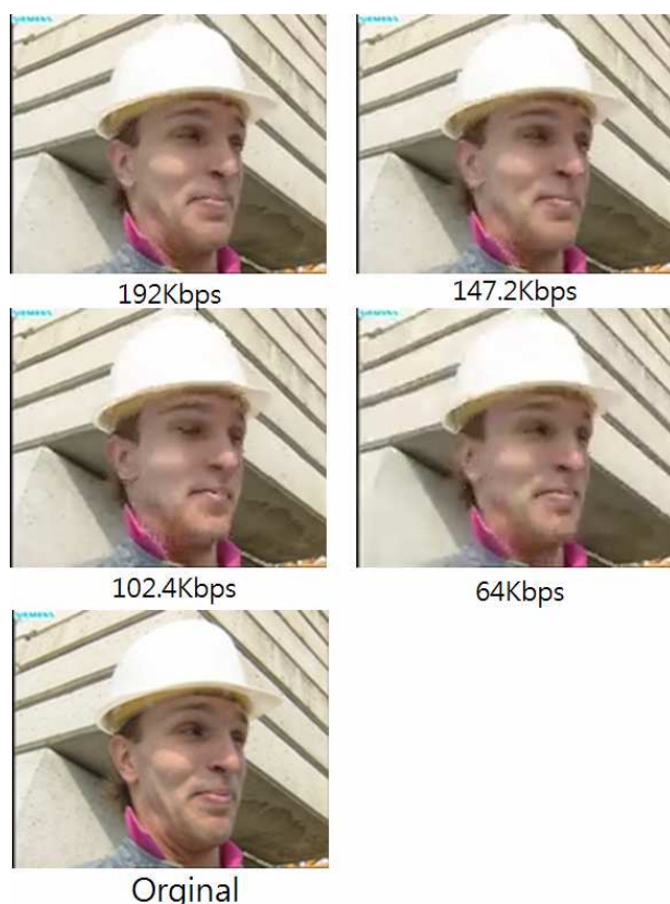
Figure 7. Comparison with 192Kbps, 147.2Kbps, 102.4Kbps, 64Kbps and original in "foreman"
