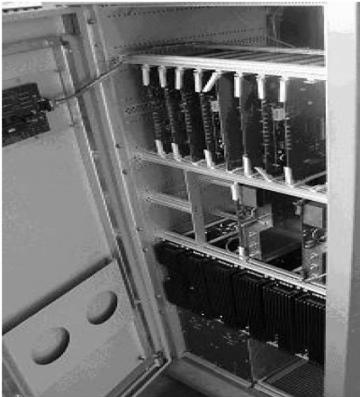
Fig. 5 Controller (the first board inner) in the cabinet
