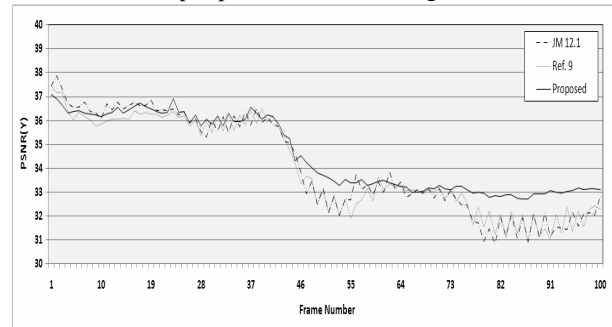
Fig. 1 Performance comparison of the proposed rate control scheme with the PSNR value per frame (Table 128 kbps, @30Hz)
