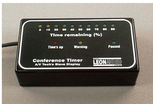
An optional unit for the A/V operator is similar in appearance to the Lectern unit. It provides a slave display without reporting any cable errors back to the Master.
