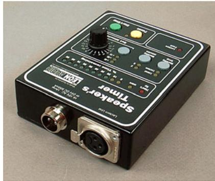
An external plug pack connects via a 2 pin locking metal connector. The plug pack can be 16-18V AC 1 amp or 24V DC at 500mA. The connector can be wired with either polarity as there is an internal rectifier. A suitable plug pack is supplied.
