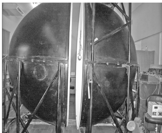
Fig. 1 NIS integrating sphere photometer system (diameter: 2.5 m)
