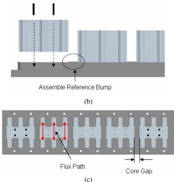
**Fig. 2** Configuration of the assembled coil block and core; (a) ISO view, (b) Side view, (c) Top view
