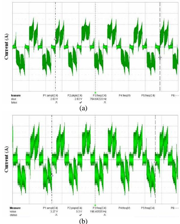
Fig. 9 Current signal measured according to driving condition; (a) no-load (b) reduction-load
