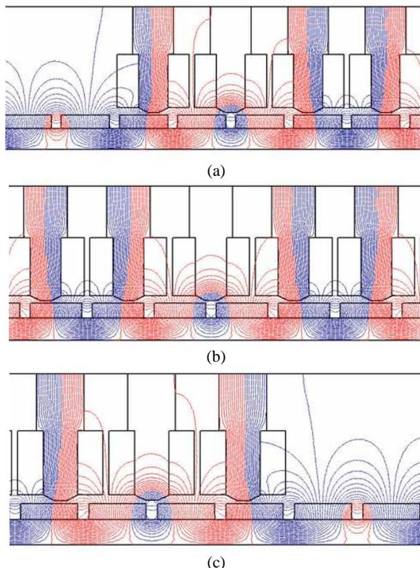
**Fig. 3** Flux distribution according to finite element model of LSM module; (a) Front element (b) Middle element (c) Rear element
