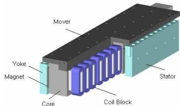
**Fig. 1** Configuration of the high-thrust and double-sided LSM module
