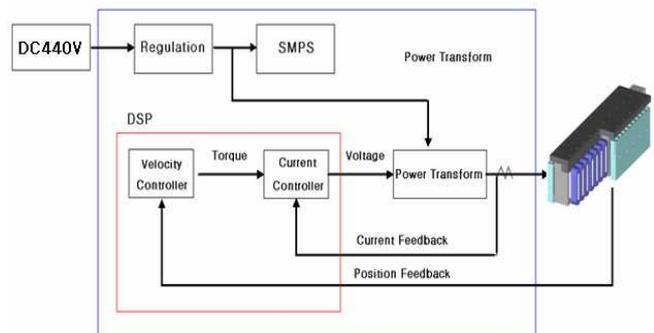
Fig. 7 Process block diagram of developed driving circuit
