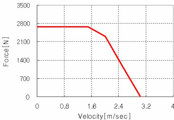
Fig. 8 Measured thrust force according to velocity condition
