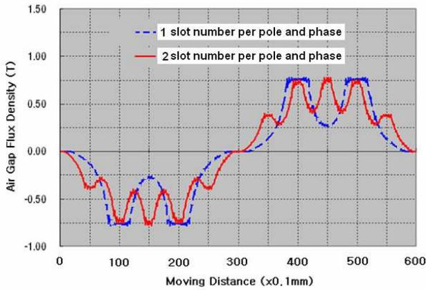
Fig. 4 Air gap flux density distribution according to slot number per pole and per phase
