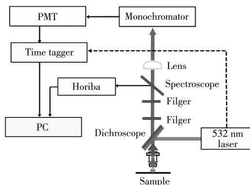
Fig. 2 Test system of luminescence spectrum and fluorescence lifetime
