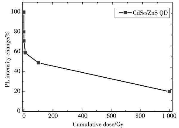
**Fig. 5** Relative change of QDs luminescence intensity plotted in percentage as a function of irradiation doses
