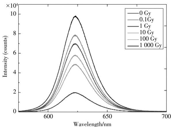
**Fig. 4** Luminescence spectra of CdSe/ZnS QDs embedded in PDMS irradiated with different doses
