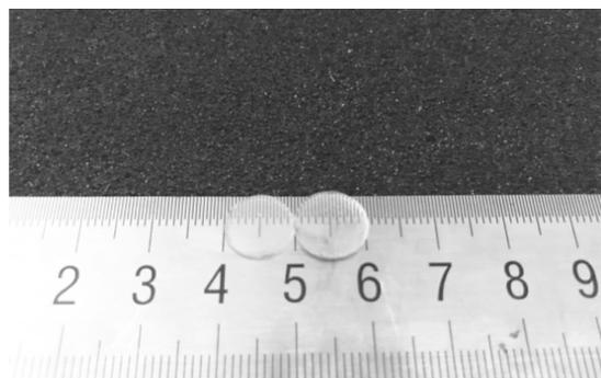
Fig. 1 Samples of CdSe/ZnS QDs embedded in PDMS
