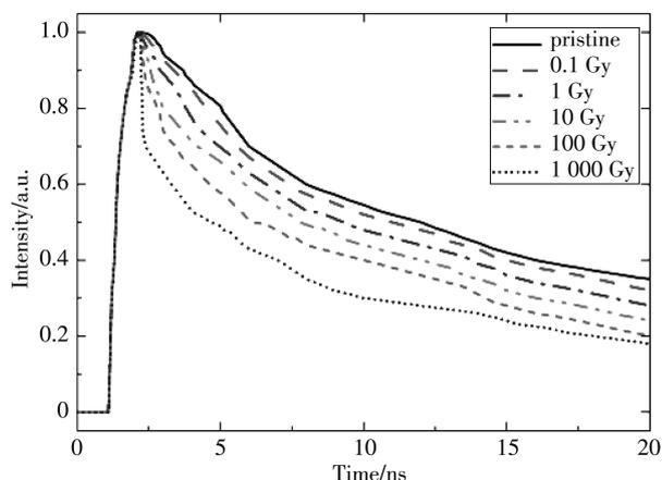
**Fig. 6** Fluorescence lifetime of CdSe/ZnS QDs embedded in PDMS irradiated with  $\gamma$ -rays at different doses
