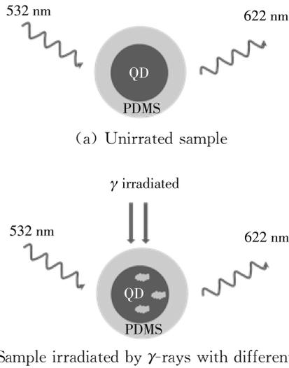
**Fig. 3** Irradiation principle of CdSe/ZnS QDs embedded in PDMS
