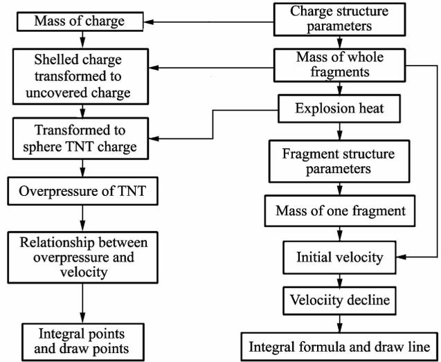
**Fig. 1** Framework of computing system of fragments and shock wave's movement
