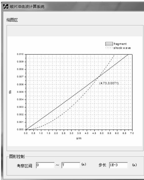
Fig. 3 Curves of time-displacement for fragment and shock wave
