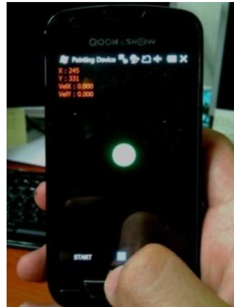
Fig. 2 A prototype of the proposed system on smartphone. The green ball expresses now relative position of smartphone.
