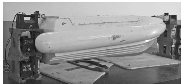
Fig. 2 Measurement setup of transverse moment of inertia
